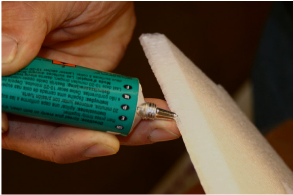
Apply a bead of UHU Por along the trailing edge of wing and the elevons
