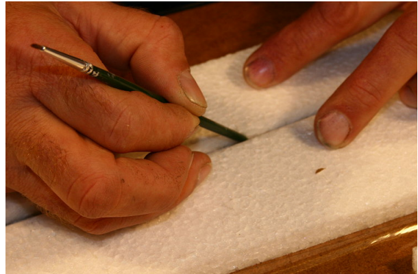
Run the end of a small paint brush along the groove to get a "U" shape fillet of glue
