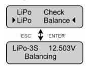
As the balancing job goes on, you can see the individual voltage by pressing 'ENTER' button. When the balancing job is completed, the beep sounds 20 times. (You can set the beep sound 'OFF' by pressing 'SELECT' button for more than three seconds. Or you can set it 'ON' by doing the job again. The default is 'ON'.)
