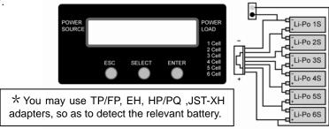
It shows the type of battery and number of cell-count at upper right, and output voltage. At lower line, it displays the residual capacity at percentage and visual graph.
