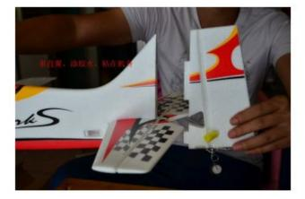
**KIT version only:** Secure control horn on the elevator. Install Z-bend wire into the hole of clear control horn clip Connect control horn clip to the servo on the elevator. Clip the control horn into the control horn clip.
