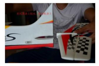
Secure the rudder into the slot on the fuselage with foam safe glue
