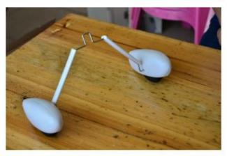
Install the assembled landing gear into the pre-cut slot on the bottom of fuselage.
