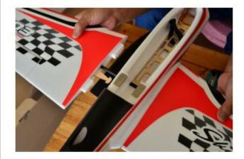
Secure the wing on the fuselage with the rubber Oring.
