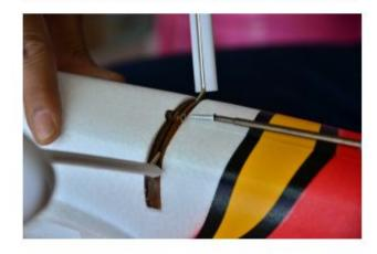
Insert main wing into the fuselage.
