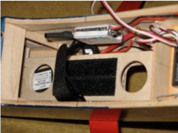
battery is velcroed to this both fore and aft and by a lateral strap.
