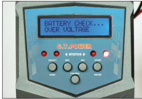
A typical alarm screen. In this case I had set the LiPo cell count wrong.
