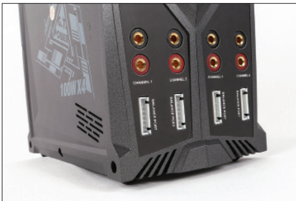
The four front charging channel outlets.
