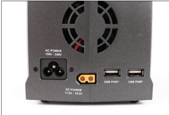
The rear sockets for AC/DC input. Note the two USB ports too.
