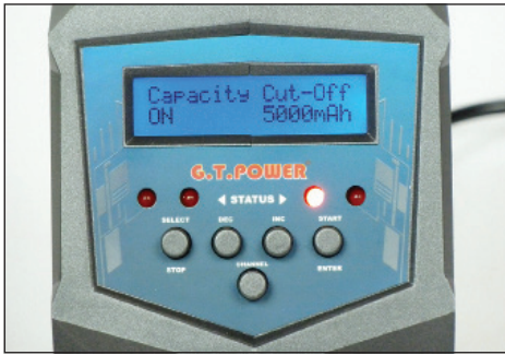
The capacity cut-off screen switches the charger channel off when the output reaches the set point.
