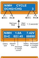
Set the sequence on the left and the number of cycle on the right. You can use this function for balancing, refreshing and break-in the battery. To avoid rising temperture of the battery, there will a brief cool-off period that already fixed at 'User setting' after each charge and discharge process. The cycling number ranges from 1 to 5.
