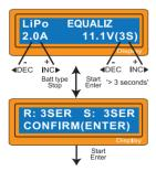
The value on the left side of second line sets a charge current and the value on the right side of second line sets the voltage of the battery pack.
