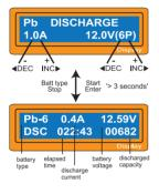
Set discharge current on the left and final voltage on the right. The discharge current ranges from 0.1 to 1.0A.
