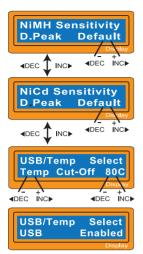
The effective value ranges from 5 to 20mV per cell .if the trigger voltage is set higher, there is a danger of overcharging the battery; if it is set lower, there is a possibility of premature termination. Please refer the technical specification of the battery.(NiCd default:12mV, NiMH default:7mV)
