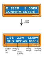
This shows the number of cells you set up and the processor detects. 'R.' shows the number of cells found by the charger and 'S: 'is the number of cells selected by you at the previous screen. If both numbers are identical you can start charging by press Start/Enter button. If not, press Batt Type/Stop button to go back to previous screen. Then carefully check the number of cells of the battery pack to charge again.
