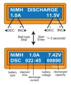
Set discharge current on the left and final voltage on the right. The discharge current ranges from 0.1 to 1.0A and the final voltage ranges from 0.1 to 25.0V). To start the process, press Start /Enter key more than 3 seconds
