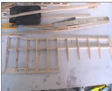
Place all ribs in position on S3
