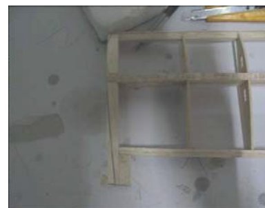
Draw a line on W 10 as shown on the plan as a guide to shape the wing tip
