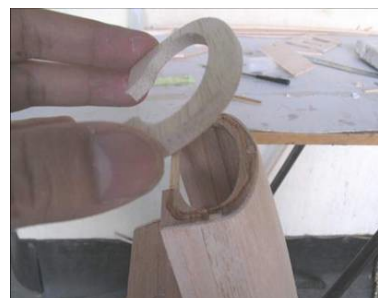
Lightly sand the front of F1 smooth and then glue F0 in position with UHU Hart
