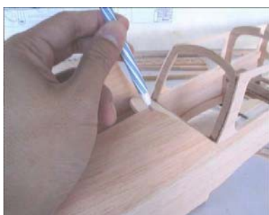
Carefully pull the sheet around the nose and glue inside the sheet with CA, and then mark where the sheet crosses the centerline of the stringer. Cut the sheet at the line you marked
