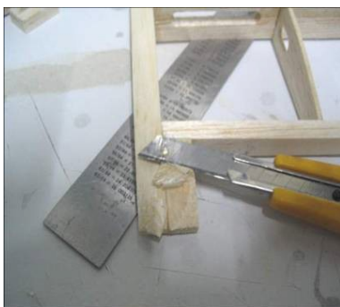
Glue S 9 in position and trim S 9 even with W 10
