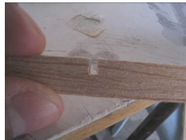
Use small flat file to file S2-S3 notches to allow the ribs fully seated on the spars
