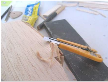
Trim flush with the side of the fuselage
