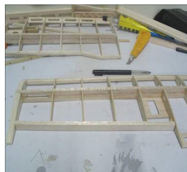
Glue S8 and S14 in position as shown on the plan
