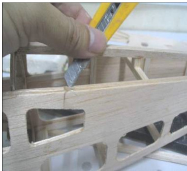
Slightly beveled P5 to fit against F16
