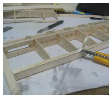
Trim S8 to match angle of the ribs (Top)
