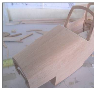
Lightly sand the nose to remove any glue
