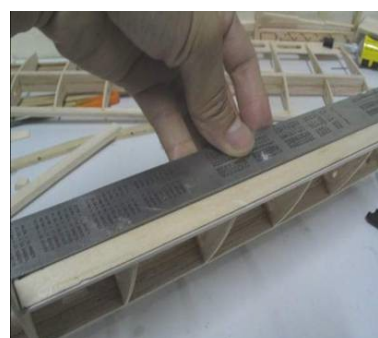
Place a straightedge against W5 and W10 and drawn a line on S8 all the way
