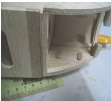
Carefully glue B3 to B2 and glue B2 to B6 with a drop of CA (attaching it to the fuselage It will be much easier to sand)
