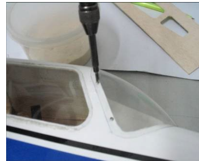
Cut the windshield on the cut line.
