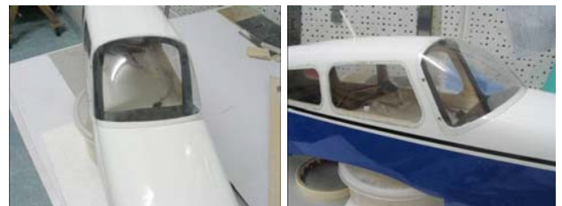
Secure the windshield in place with small sheet metal screws as shown
