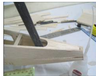
Glue a 3 mm. scrap balsa to the bottom and sand as shown
