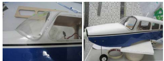
Secure the windshield in place with small sheet metal screws as shown
