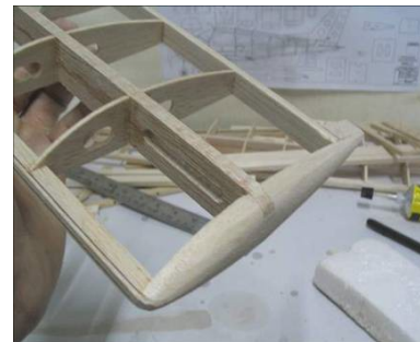
Use sandpaper to final shape the wing tip
