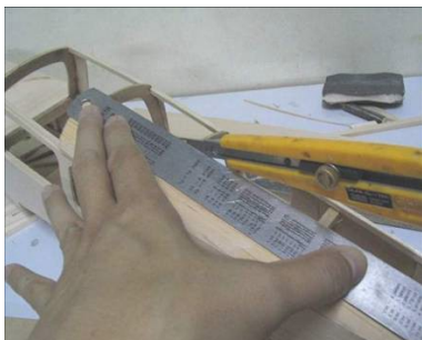
Carefully pull the sheet to the stringer and glue inside the sheet with CA, and then mark where the sheet crosses the centerline of the stringer. Cut the sheet at the line you marked. Apply the other sheet in the same manner
