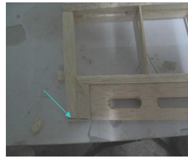
As indicated by arrow, place S10 in aileron bay and draw a line on S9 and then sand the tip to blend with the aileron
