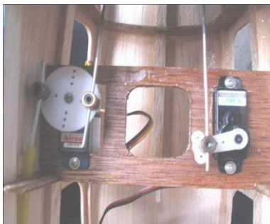
Connect the pushrod wire to the servo arm
