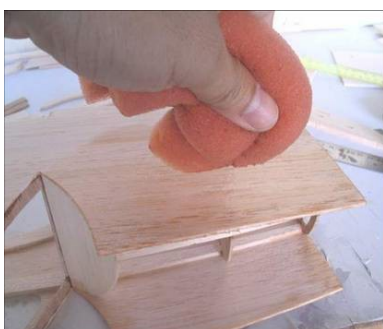
Wet outside of the nose sheet with water
