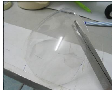
Cut the windshield on the cut line.
