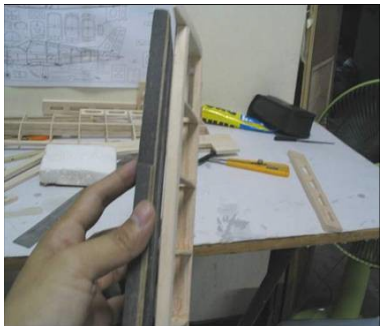
Use a bar sander to sand S8 smooth on the top and bottom
