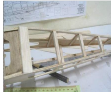
Glue P4 – F14 into position as shown on the plan
