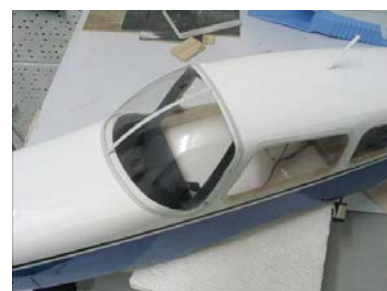
Apply silver strip tape as shown
