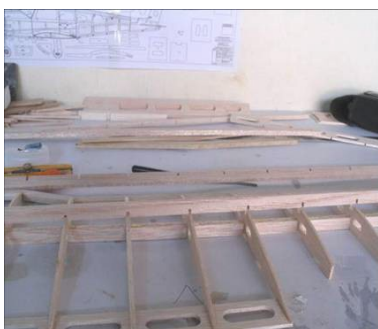
Join spar S2-S3 together
