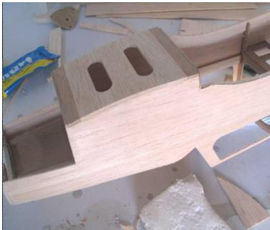
Lightly sand the edges
