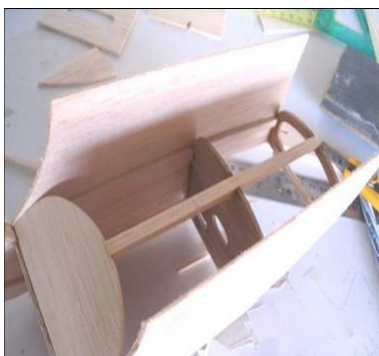
Glue F7 and P3 in position
