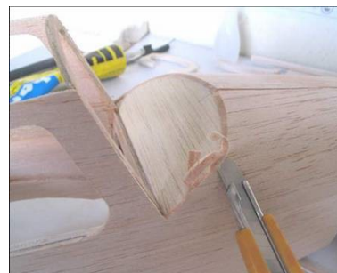
Trim the sheeting flush with F7
