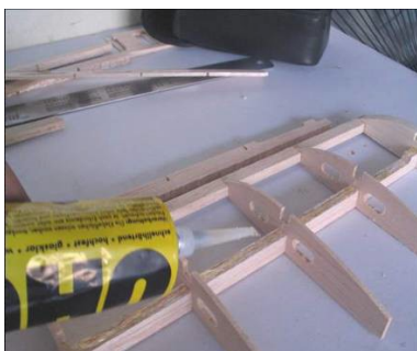
Apply UHU hart on S3 and then place S 2 into position
