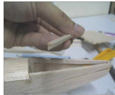
Shape a piece of P4 to triangle stick as shown
