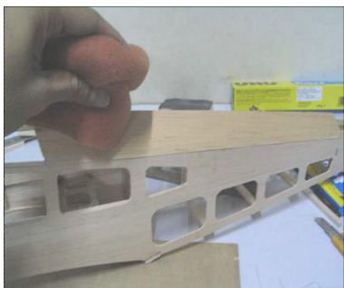
Wet outside of the rear sheet (F16) with water
