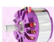
Outrunner motors are sometimes referred to as "rotating can" motors. In this design the back part of the motor (where the wires come out) is stationary and the outer can and shaft rotates. Outrunners are suited to high torque lower RPM applications like shocky's, park fliers, general sports and scale models. They throw large propellers at lower RPM which are a lot more efficient than smaller propellers at higher RPM's.
