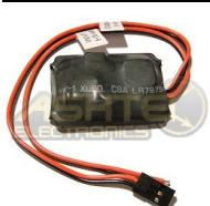
BEC is short for **Battery Eliminator Circuit** (UBEC = Universal BEC) (SBEC = Switching BEC). The BEC part of an ESC is completely separate from the circuitry which controls the speed of your electric motor.
