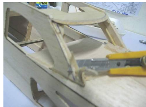
Use a cutter followed by a bar sander slightly beveled to a guideline as shown in the photo
