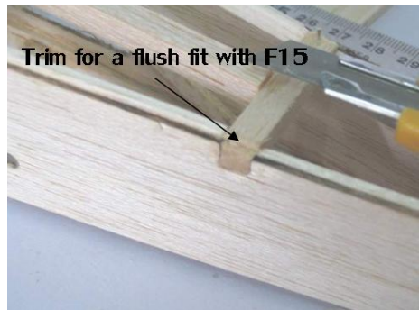
Cut a notch on P9 to fit against F15
