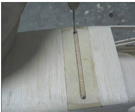
Drill 2.2 mm. pilot holes through F7 for landing gear wire as shown in the photo
