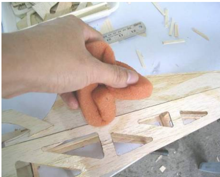
Wet outside of F15 with water
