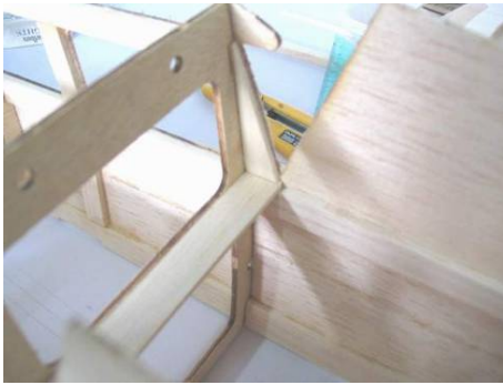
Position F12 and P7 in place
