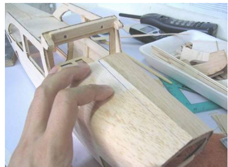
Apply the other nose sheet in the same manner
