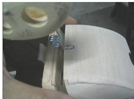
Mark the slot for Nose gear wire.
