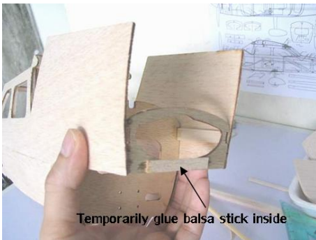
Place F1 in position (Temporarily install balsa stick inside to prevent F1 broken during holding the fuselage)
