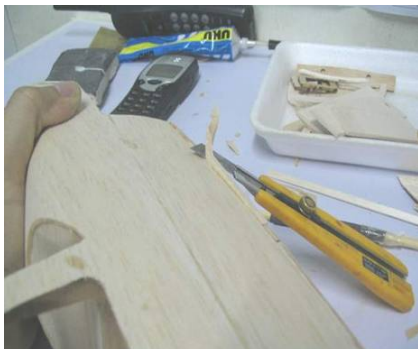
Trim flush with the fuselage
