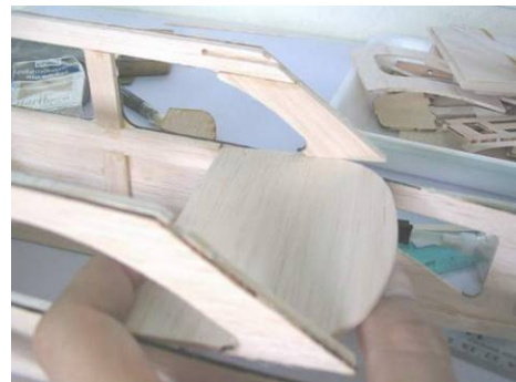
Position F13 in position as shown on the plan (Don't glue F13 to B1 yet)
