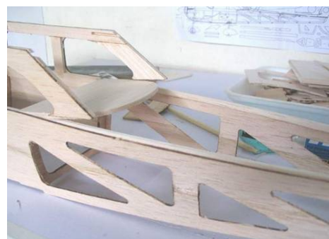
Position P8 and F6 to the fuselage frame
