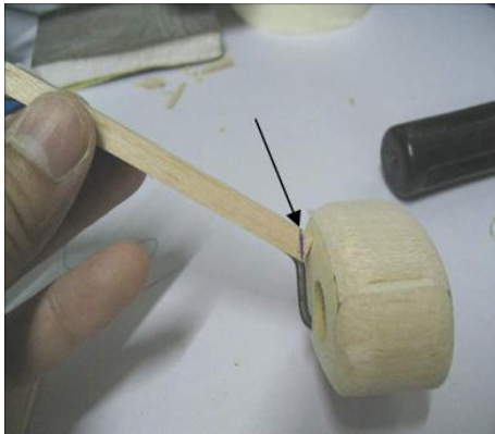
Temporarily position G1 to landing gear wire, mark and trim to the cut line to fit at the wheel pant
