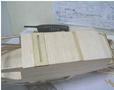
Position F7-F10 and BP2-BP4 in place. In the package, BP2-BP4 are cut lightening holes to reduce weight (BP2 smaller hole is in the front and don't glue to F9-F10 yet)
