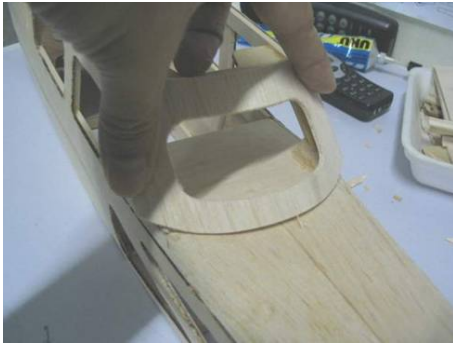
Align and glue F14 into position
