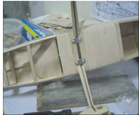
Position the main landing gear wire in place and then position the two landing gear straps over the main landing gear. Secure landing gear strap with sheet metal screws
