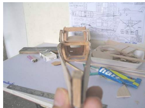
While gluing P9 in position visually center the tail to the centerline of the fuselage
