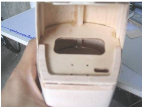
Place B4 in position, use only a spot of CA to hold it in position
