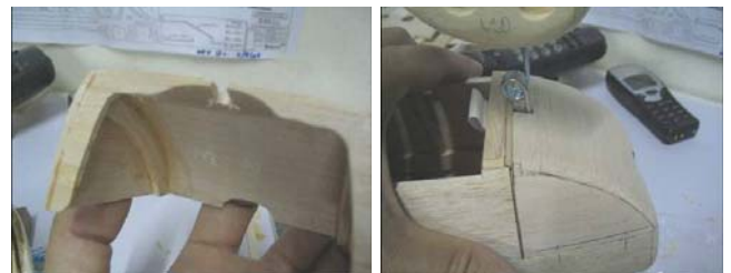
Carve a space for Nose Gear bearing and cut slots to allow the Nose gear wire to move freely. Make adjustments as necessary
