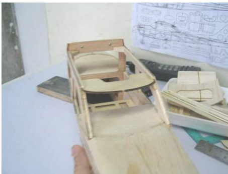
Place F15 between the fuselages sides (B1), and keep the fuselage in alignment
