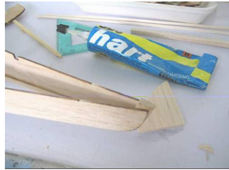
Glue P9 to the tail in position where the rear of the fuselage sides met
