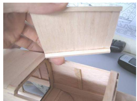
Remove battery hatch from the fuselage
