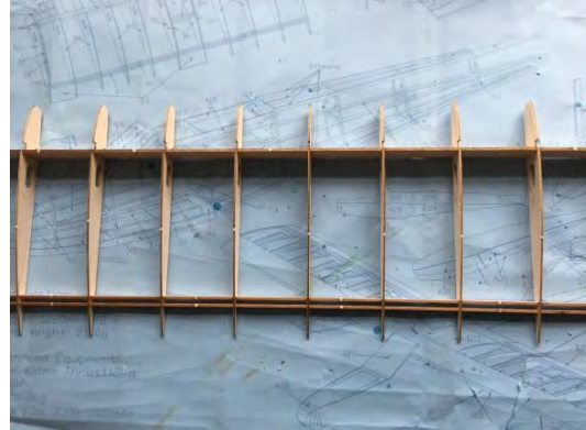
31. Position and glue to the 2 off 6x8mm main spars, wing ribs B4 and B5, B5 are the center ribs. Also add the rear spars B7 and B8.
