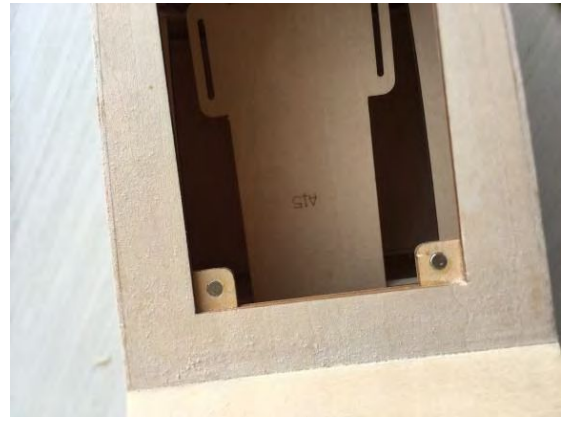
29. Glue another pair of magnets to the corresponding part of the fuselage where the battery hatch fits. Ensure the polarity of the magnets are correct so that they attract and not repel.
