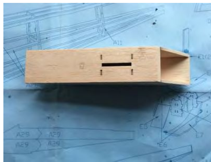
80. Form the underneath of the floats using part E7. Due to the curve these will require pinning in place as the glue dries.
