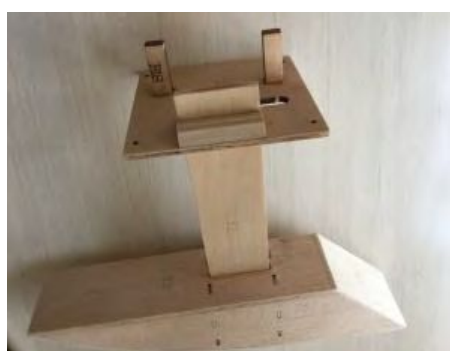
83. Glue the struts to the servo mounts exactly on the 80mm mark so that they are both identical
