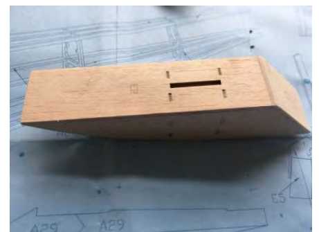
81. Cap the backend of the floats using part E5.
