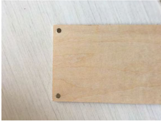
28. Glue a pair of magnets to the battery hatch part A14.
