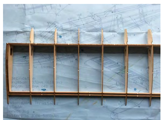
33. Add the root rib assembly that you laminated at step 30.
