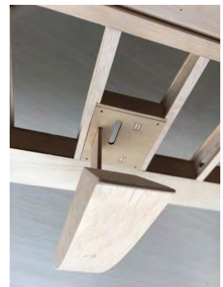
84. Screw the servo mount/float assembly to the wing.
