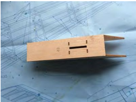
79. Add the top to the floats using part E2.
