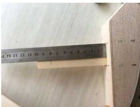
82. Glue the float struts E1 to the floats. When dry, mark a line 80mm from the top of the float onto the strut.
