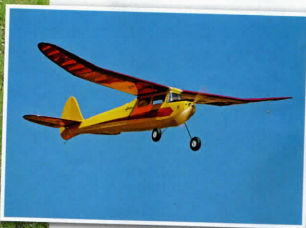
This is a simple three channel model, with wire pushrods to the rudder and elevator. Power can be electric or IC.
